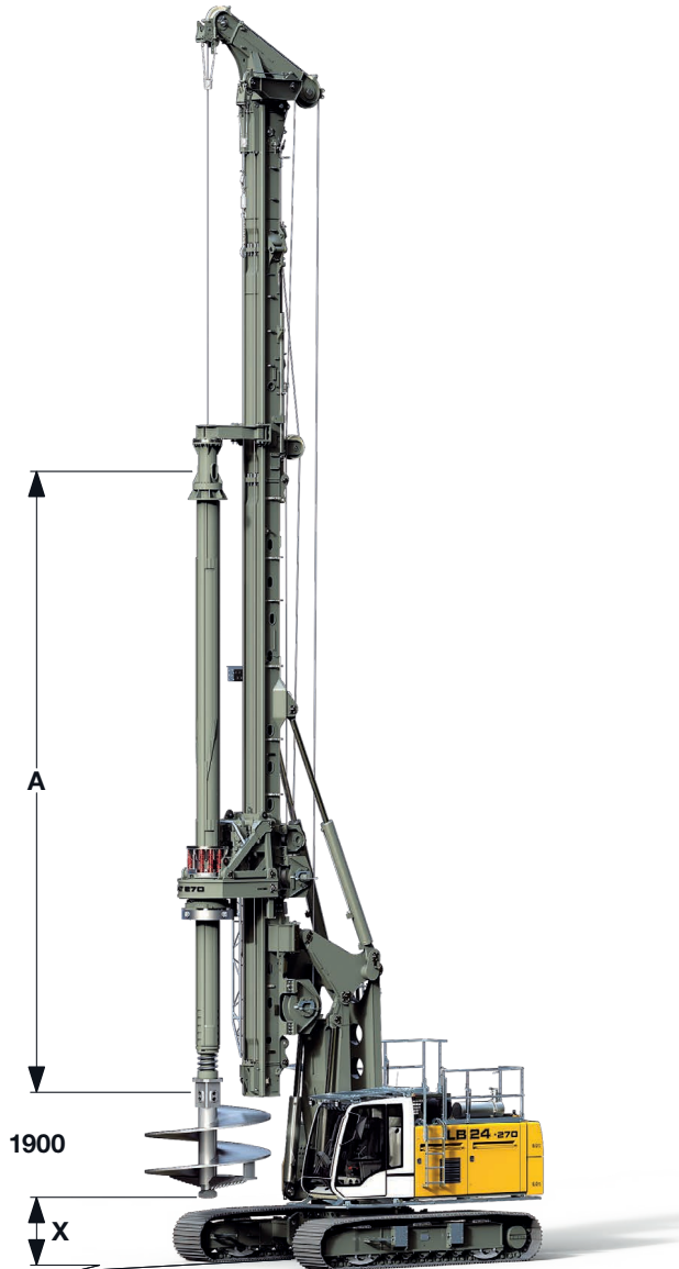
LB 24-270 with optional equipment and short leader lower part
