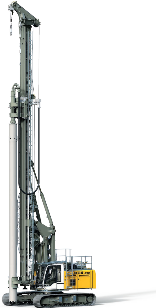
DBA 160 with protective hose
